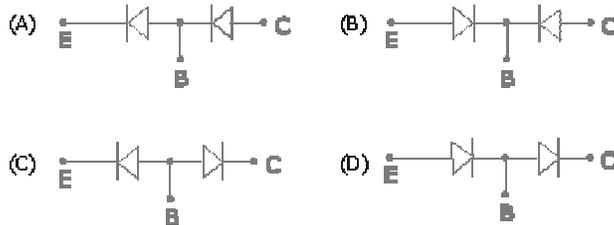
Solution: Ans (c). In transistor the emitter-base junction is in forward bias and collector-base junction is in reverse bias.
